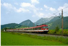
This is the train called "Transalpin". It is mainly used on the train connections Vienna–Graz and Salzburg–Graz. Its locomotive has a weight of 72 tons and stands on 8 wheels made of steel with a radius of 575 mm. The maximum load it can pull is 162 kN.
