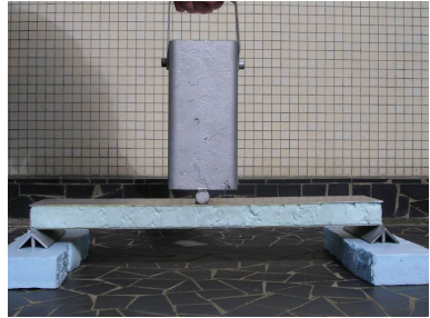
Aluminium + mousse e = 2+30+2 \text{ mm}
